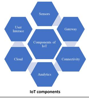
**Gateway:** For the sensors' incoming, unprocessed data to succeed in the cloud, gateways are required. Network protocols are translated by gateways, enabling seamless communication between all devices within the network. In essence, this turns the gateways into a critical communication hub and makes it possible to simply regulate data flow.
