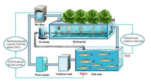
Schematic Representation of Aquaponics (Taha et al., 2022)
