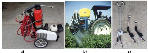
Fig. Petrol engine operated, b) tractor operated and c) different types of sprayer gun
