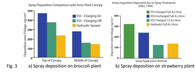
Field trials (Figure 3b) show that an electrostatically charged sprayer deposited 2.4 times more spray per leaf than a conventional high-pressure strawberry spray rig. Further trials using the air-assisted electrostatic sprayer with the charging unit turned off revealed the benefit of the air-assist feature alone: the spray deposition was 1.7 times higher than the hydraulic sprayer (Giles, 1992).
